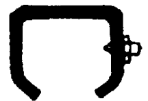
Connecting bracket #54.234 for rail #7 With set screws
